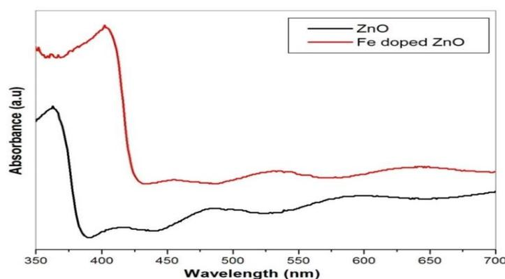
Figure 2: Optical absorption of ZnO and Fe incorporated ZnO
