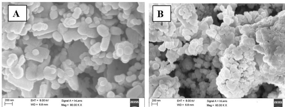
**Figure 3:** Surface morphology of ZnO (A) and Fe doped ZnO (B)
