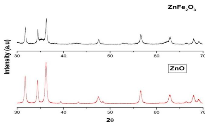
Figure 1: X-Ray diffraction pattern of ZnO and Fe incorporated ZnO
