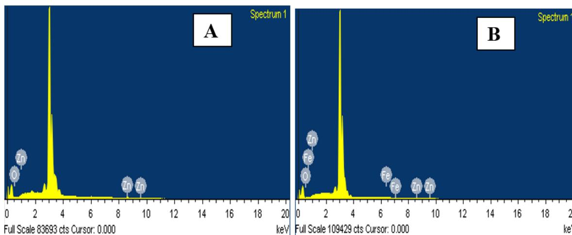
**Figure 4:** Energy dispersive spectra (elemental composition) of ZnO (A) and Fe doped ZnO
