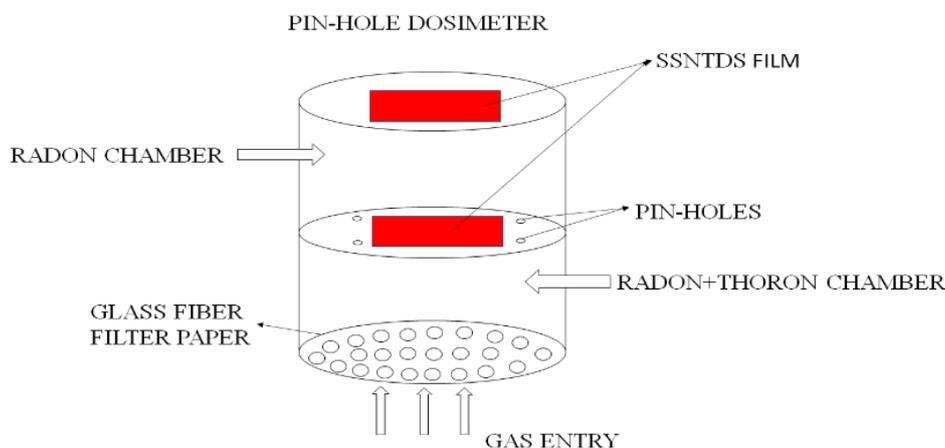
Fig.2: - Internally diagram of pin-hole dosimeter
