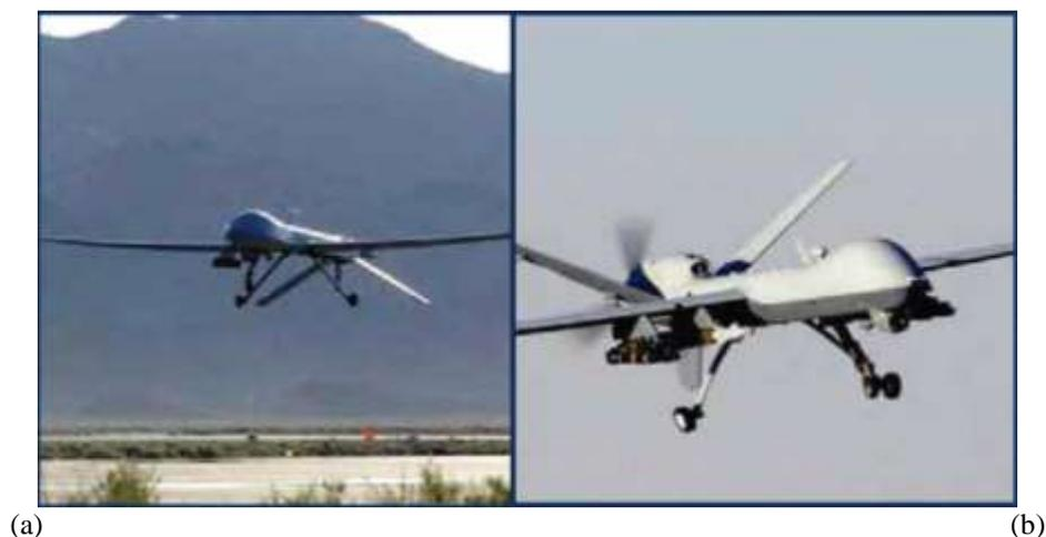
**Figure 9:** (a) MQ-1 predator and (b) MQ-9 reaper
