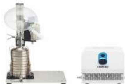
Fig. 4: Anderson Cascade Impactor (ACI)
