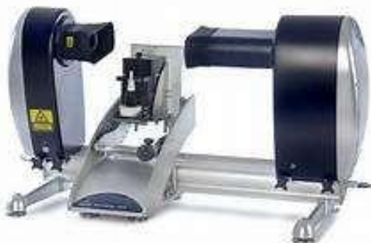
Fig. 2: Laser diffraction set up for nasal spray analysis
