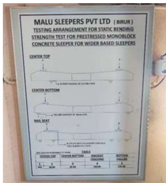
Fig 10: Testing arrangements for Static Bending Test
