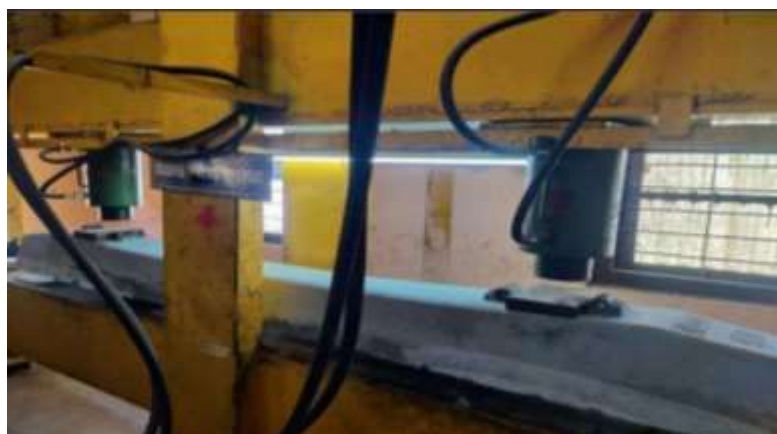
Fig 12: Centre Top Method in Static Bending Test
