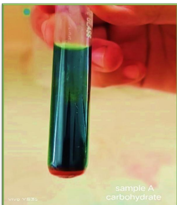
Figure 5. Test for Carbohydrate (Red Precipitate are show the presence of carbohydrates).
