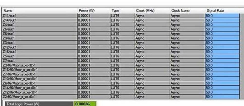
Fig. 33 Logic Power for 16-bit Reversible qALU
