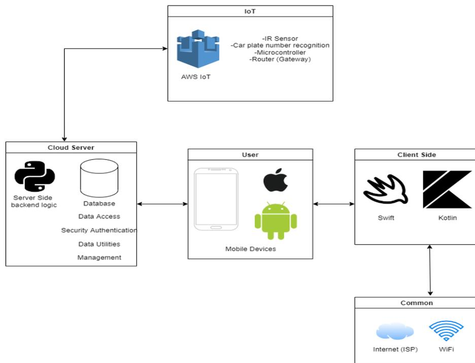
**Figure 1** shows the application's architecture diagram which utilizes IOT technology, cloud server, client and user side
