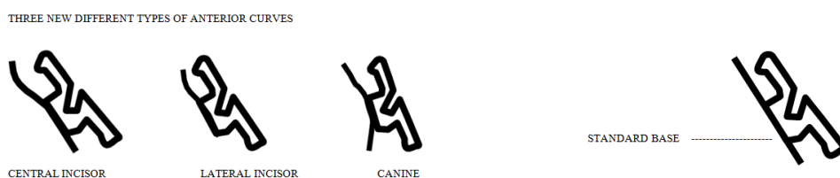
Figure 9. Customizing the design of the bracket base by following the contour of individual lingual tooth contours
