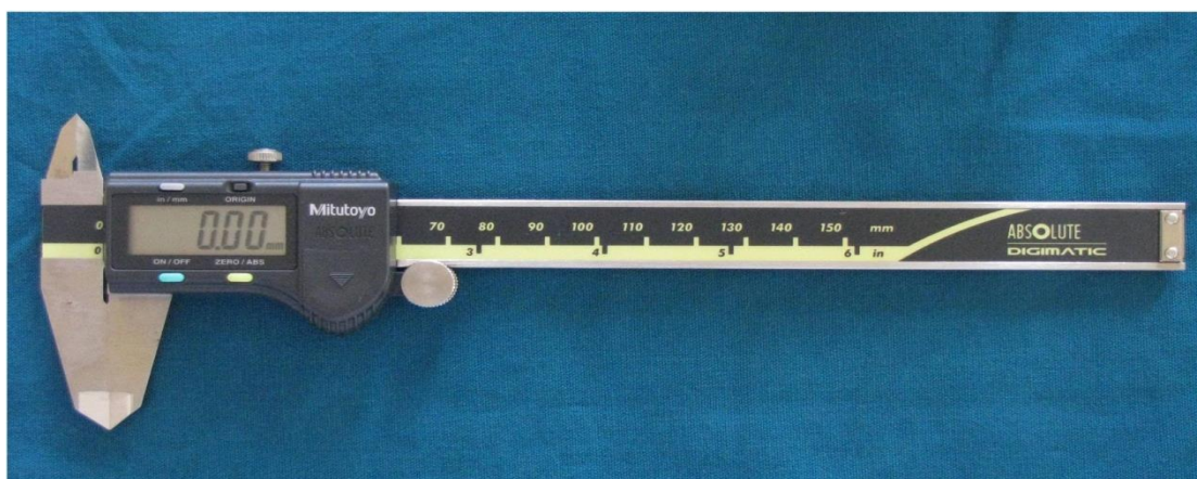
Fig.1: Electronic digital caliper accurate to 0.01 mm. (Mitutoyo Digital Caliper, Japan).
