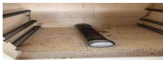
Figure(2) : An iron reactor for making rue powder Peganum harmala at a temperature of 550 C
