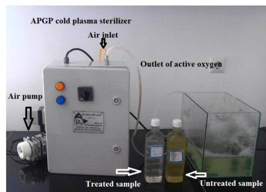
**Figure 2: Injection of active oxygen to studied samples.**
