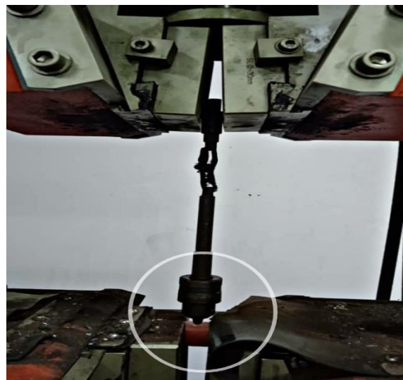
Figure No. (7) The head used to fix the post and transmit force.
