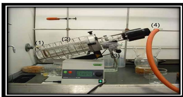
Fig. 2: Vacuum Distillation Apparatus
