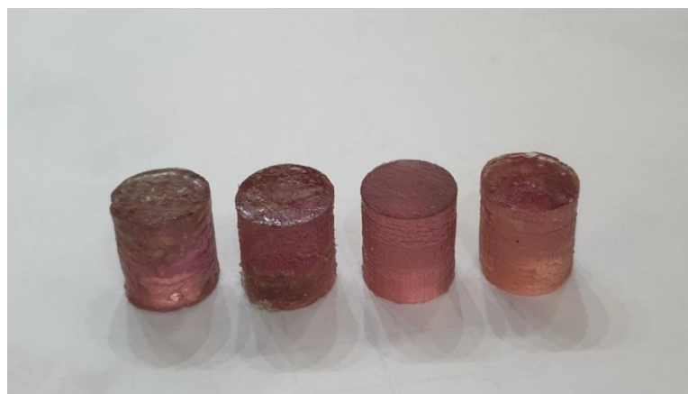
Figure 4: Shows the shape of the sample prepared for compressive resistance testing
