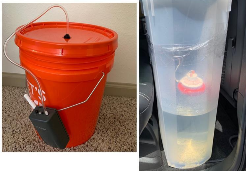
Figure 1: The two containers used in this study; container one (A), and container two (B). Both pictures depict the portable battery powered aerators used for the duration of the experiment. Not depicted in these photos are the media bags containing 0.5 cups of carbon which were used to assist with chemical filtration.
