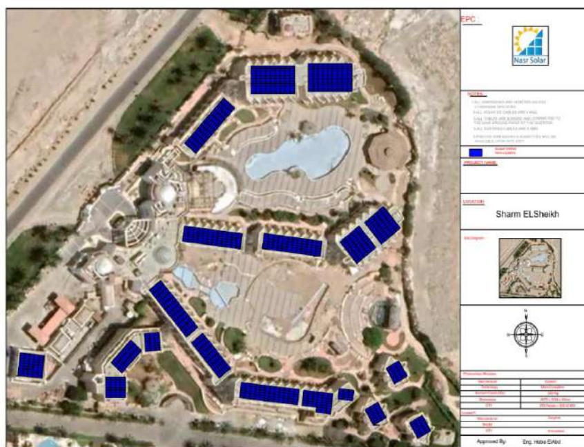
Figure 19 shows the layout of the 562 kW On-Grid system station at the first hotel
