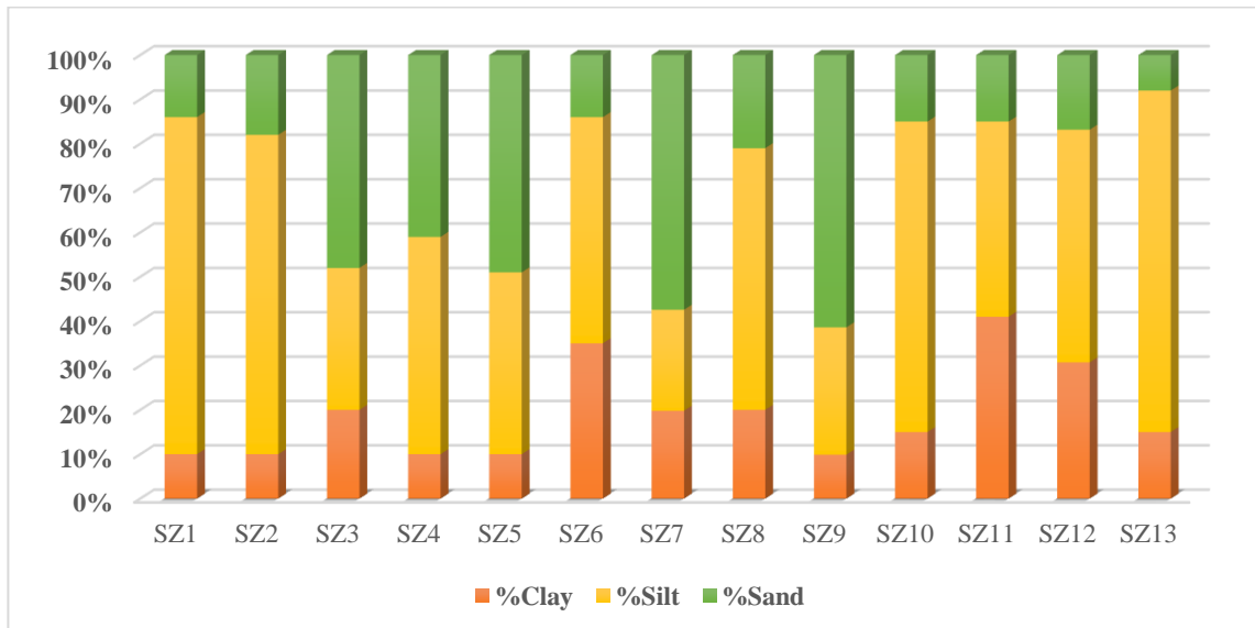
Figure 15. Percentage of clays, silts and sands in study area soils
