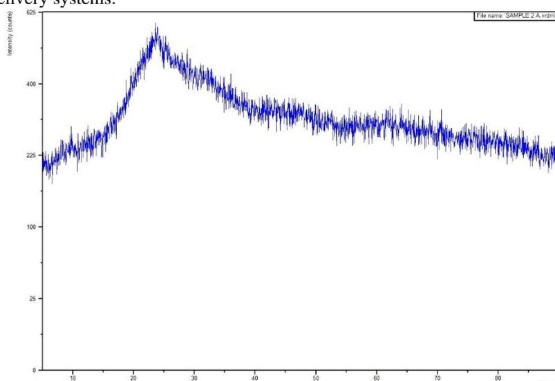
**Fig. 6. XRD graph of amorphous silica**
