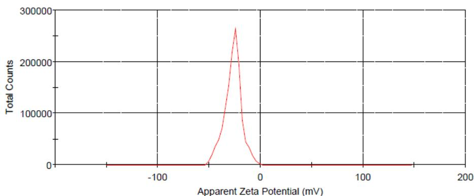
**Fig. 5. Zeta potential of amorphous silica**
