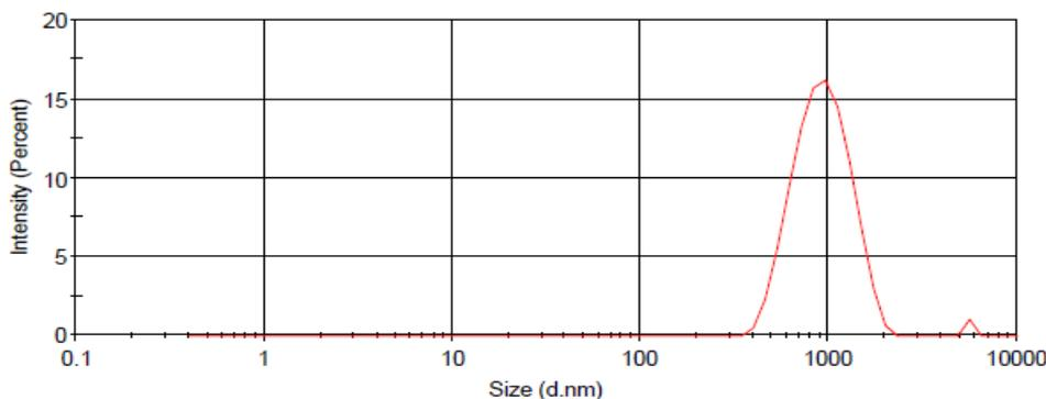
**Fig. 4. Size of amorphous silica**
