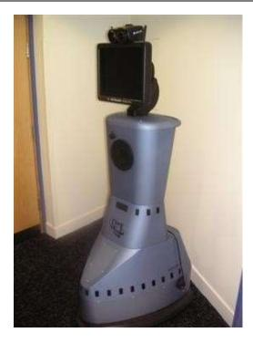
This robot is controlled remotely by a doctor, whose face appears on the monitor which acts as the robot's 'head'. This is taking telemedicine a step further because one can make the consultation 'patient-centric'. The doctor's control centre has a double screen, webcam and joystick for controlling the robot. As well as being used for patient consultations, the device can help with mentoring and training medical staff remotely.
