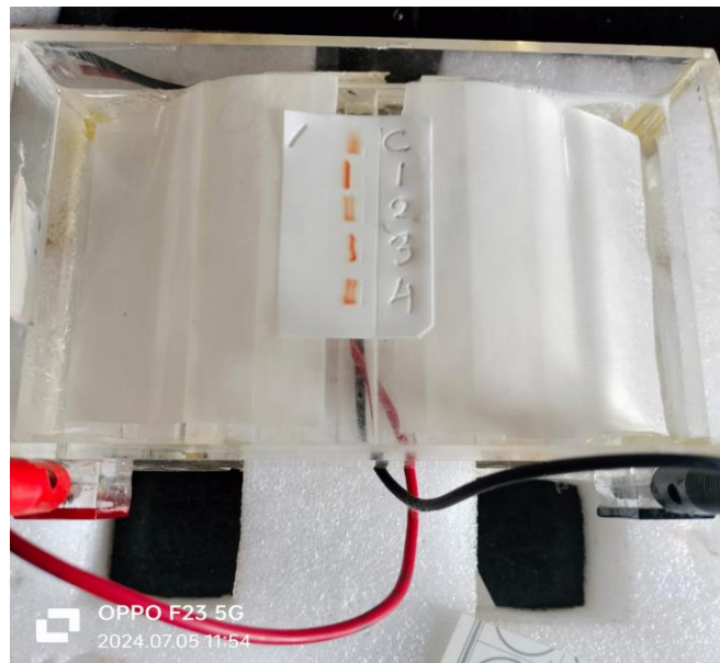
Figure 2: Real-time electrophoresis instrument SCD testing of 4 samples at a time
