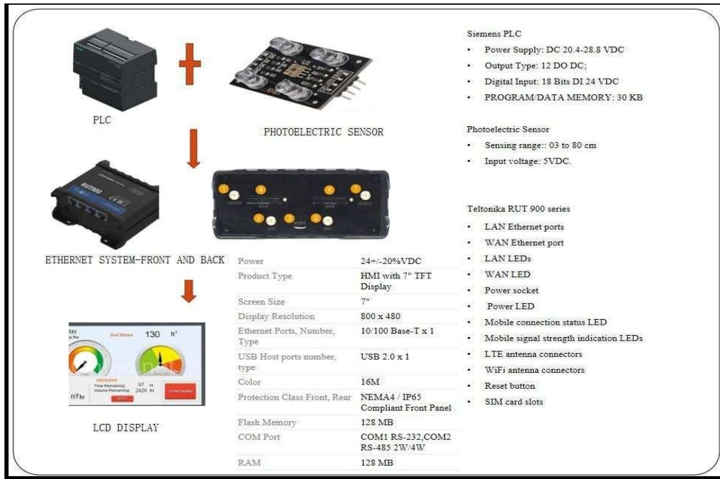
Figure 2. The hardware assembly of the developed system
