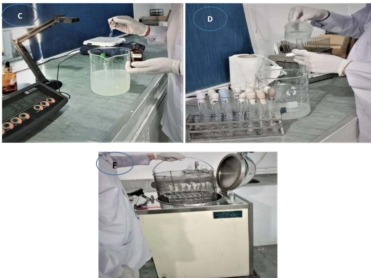
Fig. 1 Pictorial presentation of media preparation (A-preparing glassware, B-weighing MS media and sucrose, C- pH adjustment of media, D- pouring media in test tubes after dissolving agar, E-autoclaving media
