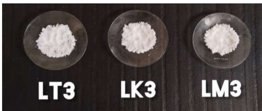
FIG 3: LOW SODIUM SALTS PREPARED USING METHOD III
