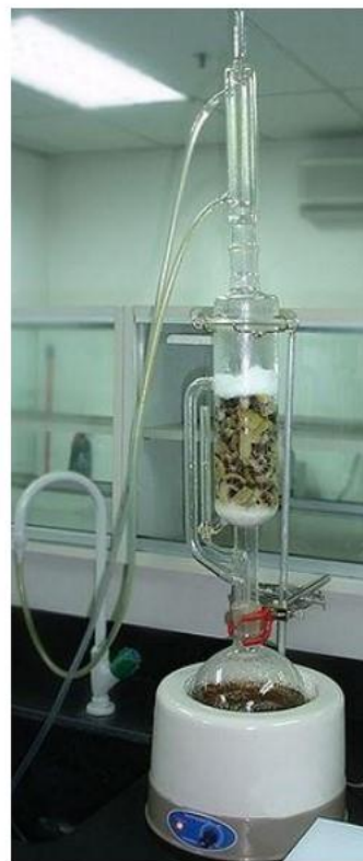
Fig 1: Soxhlet extraction setup
