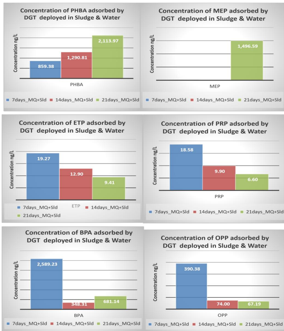
Figure 7: Time Weighted Average Concentrations (ngL -1 ) of chemicals in sludge cakes adsorbed by o-DGT in MQ water & Sludge mixture without the inhibitor NaN 3
