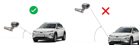
Fig. 9: Ideal position for camera angle
