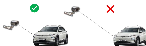
Fig. 8: Ideal position for camera distance
