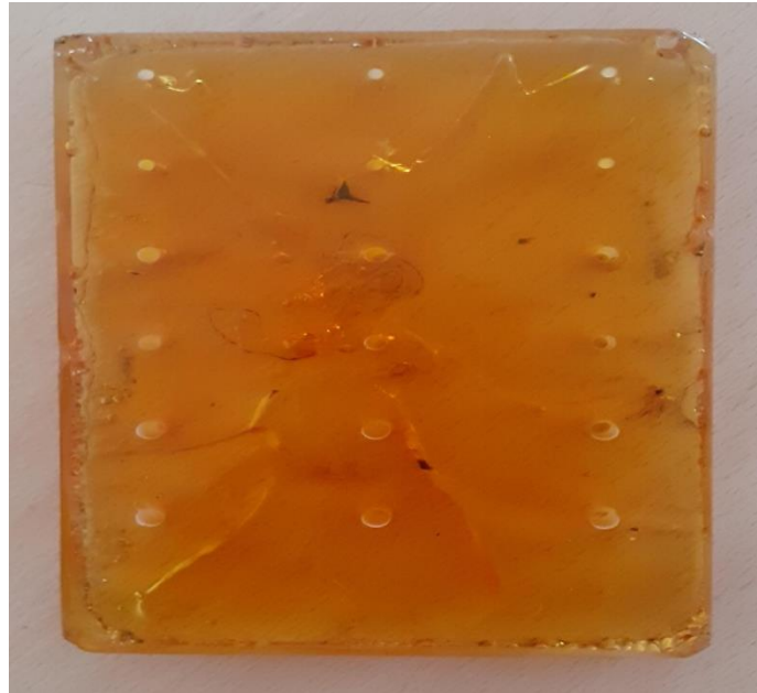
Fig. 1. CNC drilling on plain epoxy (Group 2)
