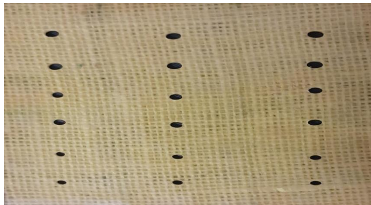
Fig. 2. CNC drilling on fiber reinforced epoxy (Group 1)
