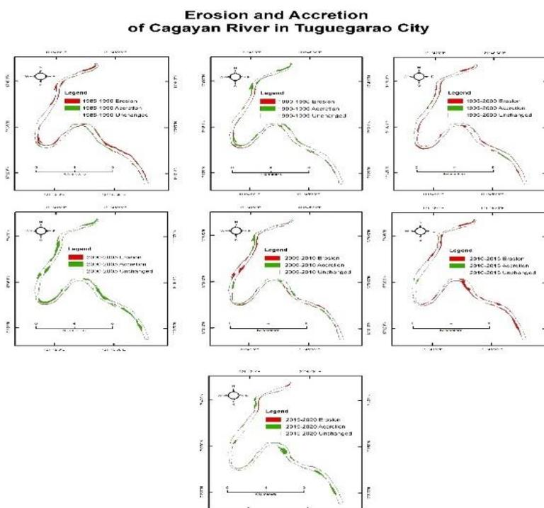
**Figure 3** Error! No text of specified style in document..7. Areas of Erosion and Accretion along the Cagayan River Section in Tuguegarao City from 1985 to 2020.
