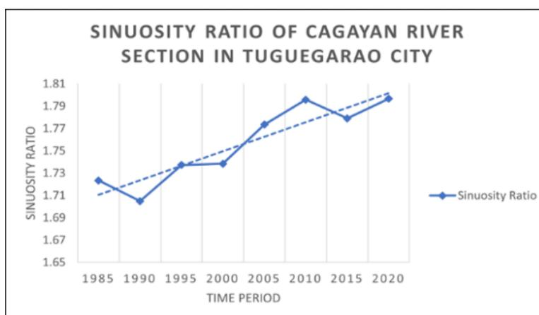
Figure 3.1. Variations in the Sinuosity Ratio of the Cagayan River Section in Tuguegarao from 1985 to 2020.
