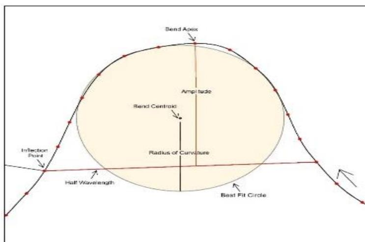
**Figure 2.1 Meander bend parameters created using ArcMap.**
