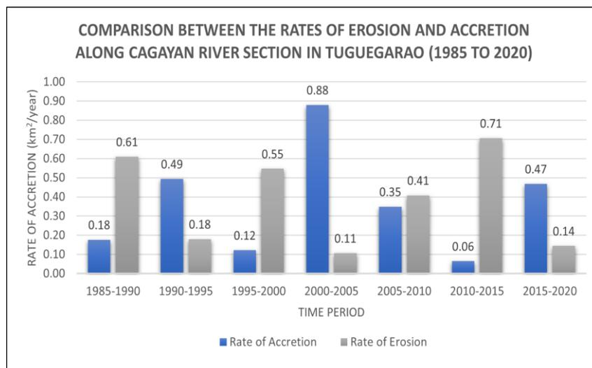
**Figure 3.3 Comparison Between rates of Erosion and Accretion along Cagayan River Section in Tuguegarao City from 1985 to 2020.**
