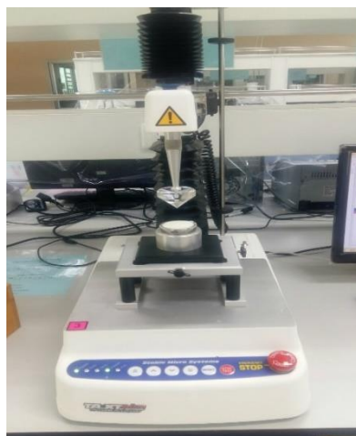
Figure 3: This picture shows the spreadability testing of the natural extracts lotion formulations using Texture Analyzer (stable micro system series-TA.XT Plus, UK)
