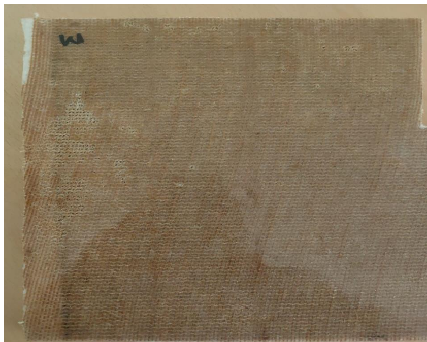
Fig. 1. Laminated plate of flax fiber and polystyrene foam structural insulated panel reinforced with wire mesh(Experimental group)
