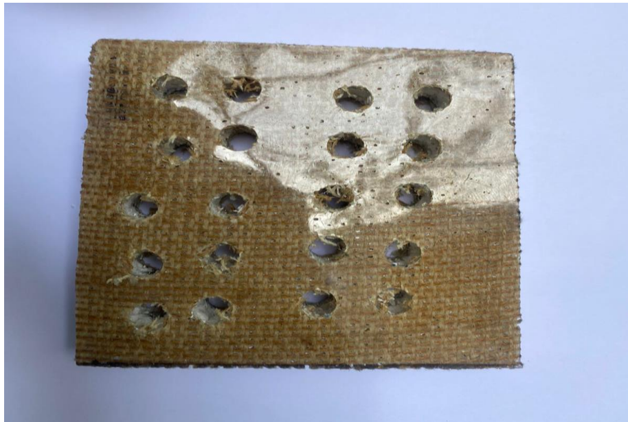
Fig. 2. Laminated plate of flax fiber and polystyrene foam structural insulated panel reinforced composite (Control group)
