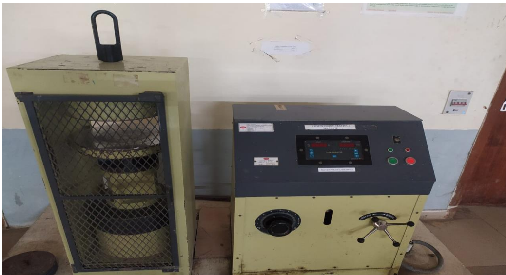
Fig. 3. Compression testing machine used to collect the compressive strength data.
