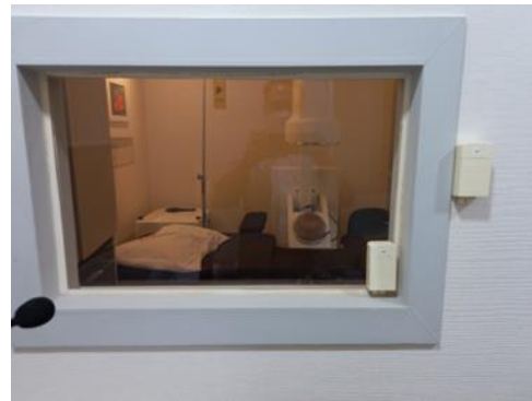
Figure 3. Glass dosimeter installed in the patient view window
